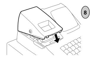
If the printer is used for journal, simply attach the Printer Cover. The Receipt Outlet is used as Journal Window.
